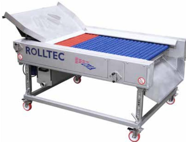
The ROLLTEC is a sorting table with rollers made by C.M.A. for the separations of the grapes from MOG - stems, leaves, little unripe or dried grapes and other external items. The ROLLTEC has a vibrating hopper on the inlet side of the machine which conveys the grapes onto the sorting rollers.
