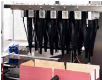
Centering funnels for a cases with preglued partition
