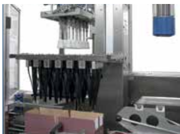
Centering funnels for cases with preglued partitions
