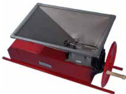
10F07 HAND CRANKED DESTEMMER Agitator, Hopper, Double Rollers, Stainless Steel.
