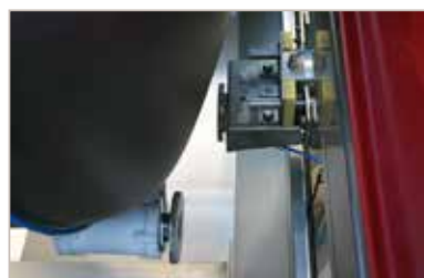
Connectors at the drum and the press frame – interrupted connection
