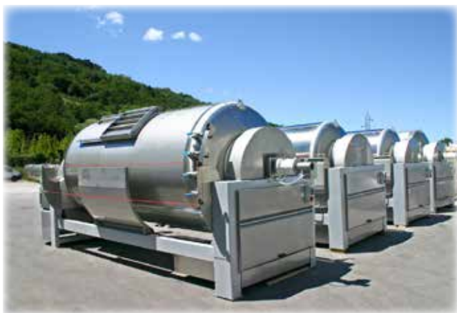
Drum design PST with connected draining channels, big draining surface
